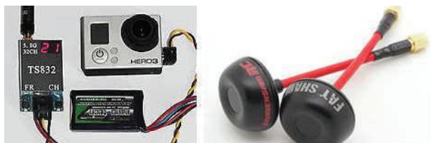
Figura 5 - GoPro, transmissor Boscam e antenas Fast Shark.
