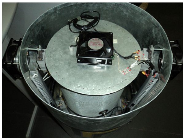
Figure 1. The grain silo prototype a view from the top of (without the roof).
