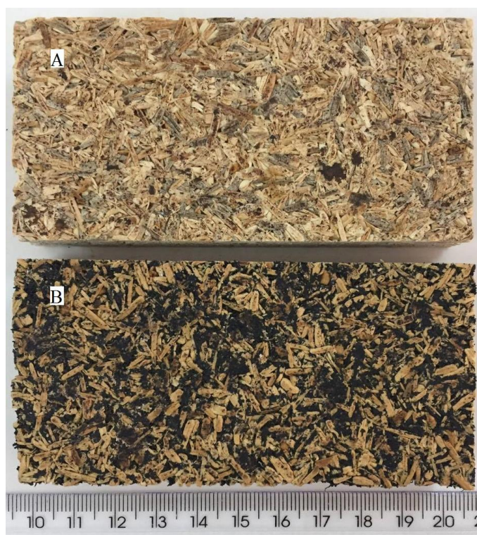
Fig. 2. Wood panels. (A) Only wood particles; (B) 30% rubber particles
