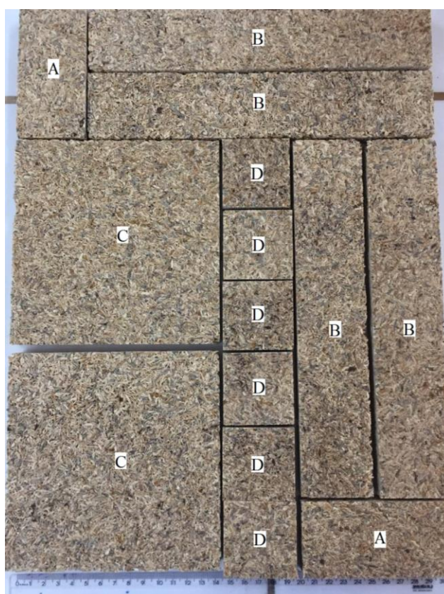
Fig. 1. Specimens in the panel. (A) Apparent density; (B) Static bending; (C) Water absorption; (D) Internal bond strength and Moisture
