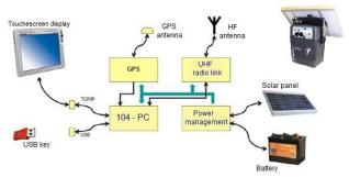
Fig. 4. General architecture of the base station [9].
