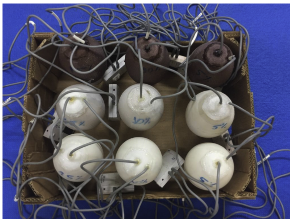
Fig. 1. Artificial fruit with skin of acrylonitrile butadiene styrene (ABS) in two colors (White ABS or Crystal ABS) (bottom or middle rows, respectively) or skin of poly lactic acid (PLA) with 5% wood powder commercially called PLA Wood (top row) with flesh containing 5, 10 or 15% of agar (right to left) placed in a cardboard box with dimensions of 38, 27, 14, and 0.12 cm for length, width, height and thickness, respectively.
