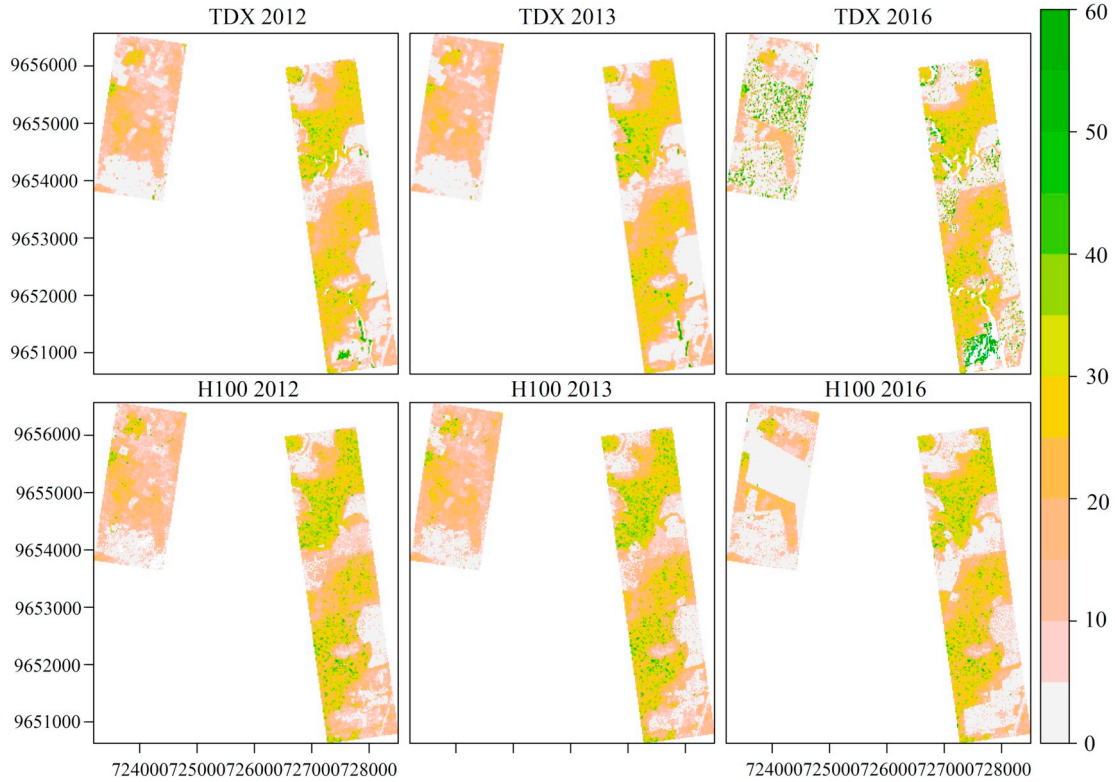
Fig. 6. Interferometric heights derived from TanDEM-X (top panel) and H100 (bottom panel) derived from LiDAR CHM, for 2012, 2013 and 2016. For each year and sensor, the two rectangles correspond to the LiDAR coverage.
