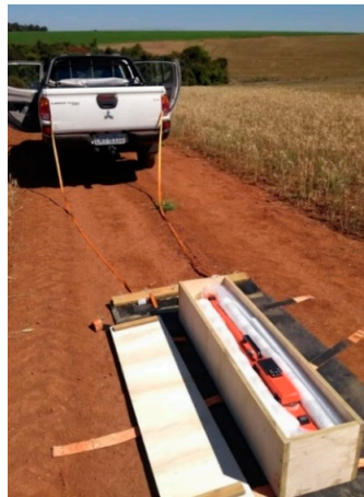
Figure 2. Mobile data acquisition structure for EM38-MK2 on-the-go survey.
