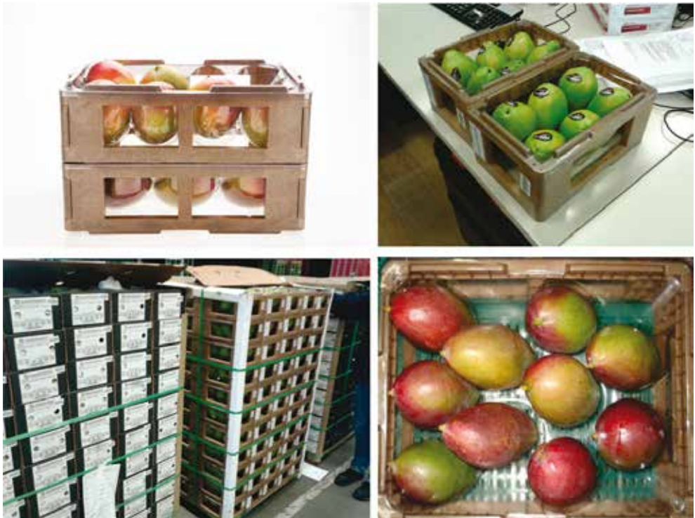
Figure 2. Packaging designed for papaya and mango that reduces losses.
