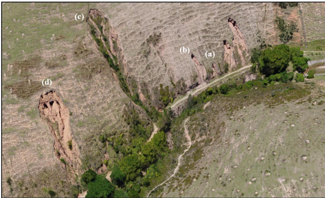
Figure 2. Gullies in different stages of formation. (a) Gully in the initial stage; (b) gully in the juvenile stage; (c) gully in the senile stage; (d) gully in the mature stage.
