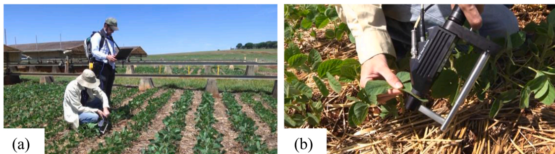
Fig. 2. Spectral assessment in the field (a) and detailed view of the plant probe device (b). Photo by Décio de Assis – Embrapa Soja.
