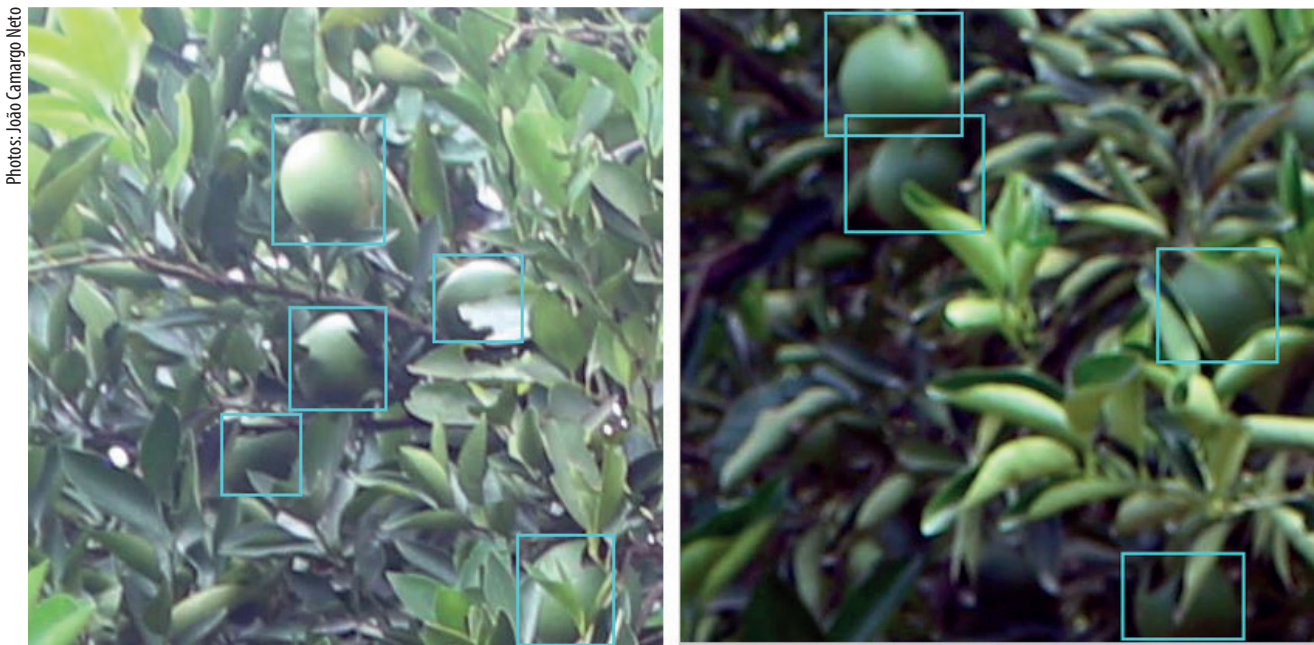
Figure 3. Examples of the difficulties faced in fruit detection. In the images, we can observe problems of focus, specular reflection, severe occlusion by leaves, branches and other fruits, light variations and similarities in the color pattern between fruits and leaves.
