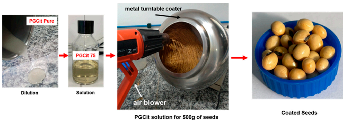
Figure 2. Soybean coating procedure with PGCit polymers.
