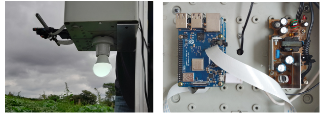
(a) Details of the camera, stereo rig and lamp. (b) Interior of protective case, with RPis and rectifier.
