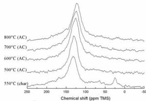
**Figure 2.** <sup>13</sup>C SPE-MAS NMR of the charred precursor and the activated carbons (AC) prepared at different activation temperatures using  $H_3PO_4$  as the activating agent.
