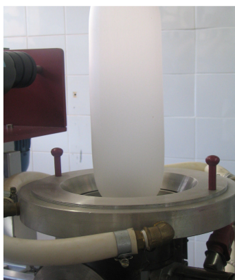
Figure 1. Lipophilic starch bioplastic being formed by blowing.
