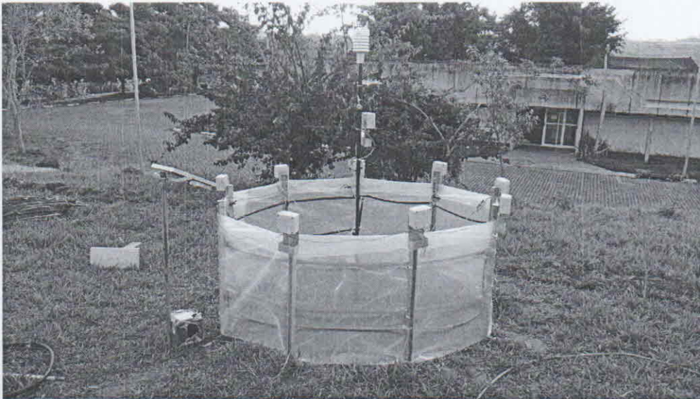
Figure 3 – The OTC experiment instrumented with the ZigBee based wireless devices.
