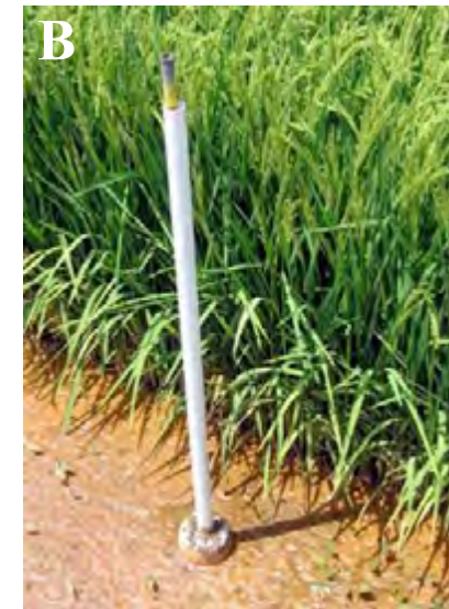
Figure 6. Overhead sprinkler irrigation of rice in Arkansas (A). Simple depth gauge consisting of seine float attached to PVC pipe being used to help manage rice flood (B). (Sprinkler rice photo credit: Dr. Brian Ottis, RiceTec.)
