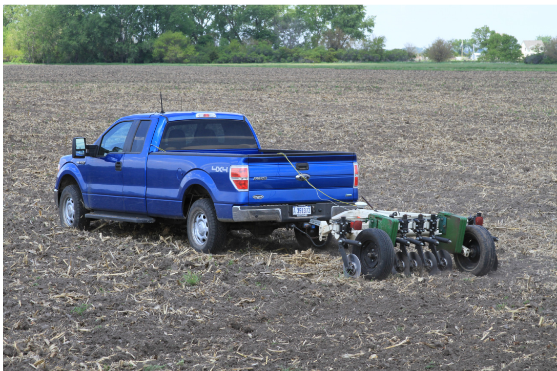
Appendix 3.2. Real Time Kinematic GPS base station and equipment to measure EC (Veris). Source: (ARS/USDA server).
