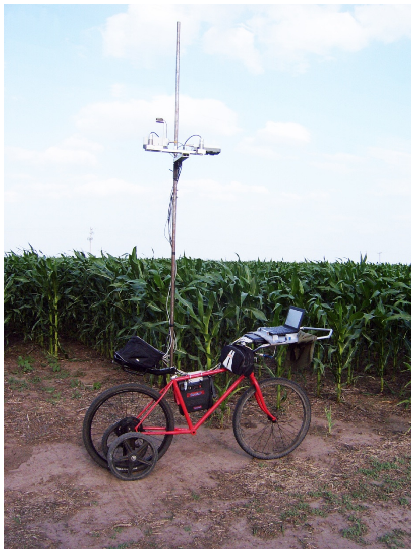
Figure 1. Platform for data acquisition (bicycle equipped with 2 optical sensors, DGPS, laptop computer and batteries).
