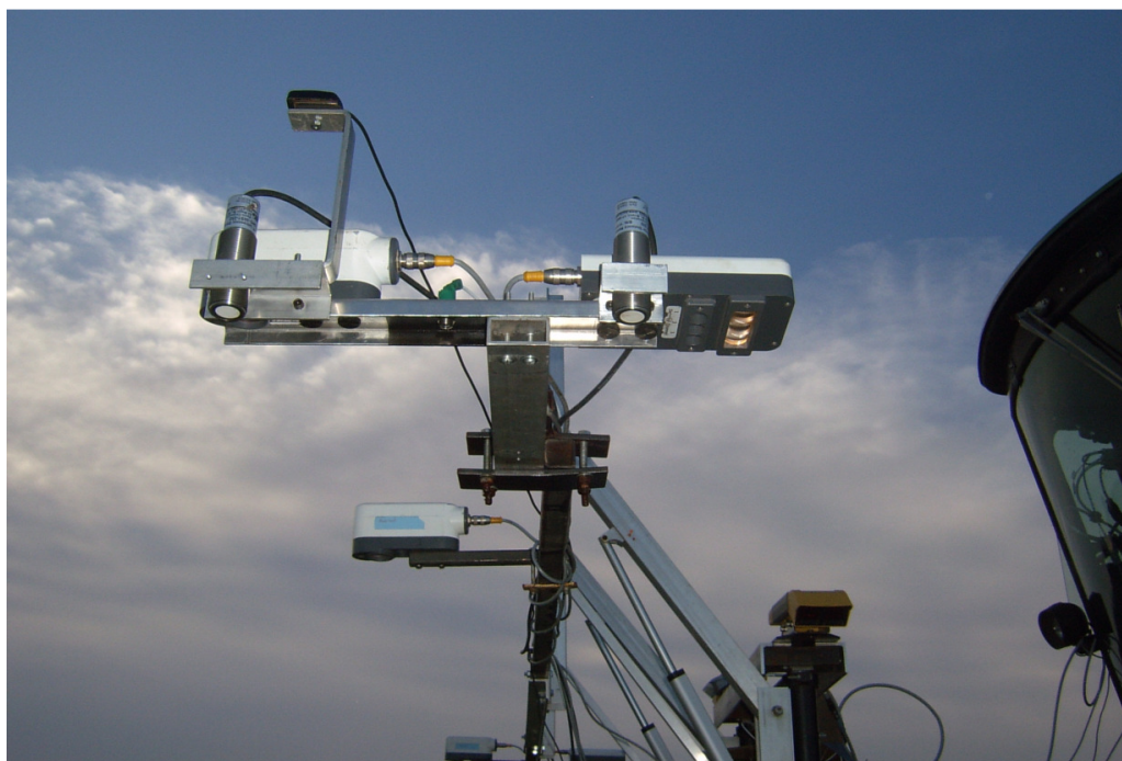
Appendix 3.1. High clearance machine used to take sensor readings and the sensor attachment to the spray boom.
