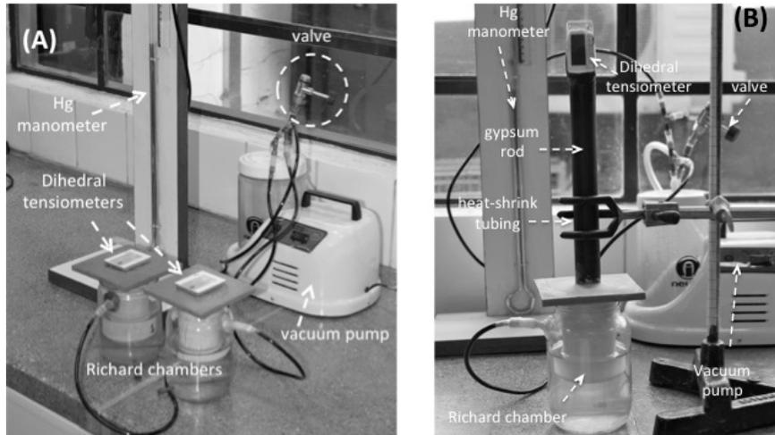
Fig. 4. Experimental setup to test the dihedal tensiometers S1, S2 and S3 (A) and the glass/glass dihedal tensiometer (S3) connected to a gypsum rod shown in Fig. 3 (B).
