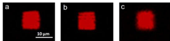
Fig. 14. Confocal microscopy images of planes of cubic structure containing rhodamine, fabricated by TPA polymerization. Images from (a) bottom, (b) 6.0  $\mu\text{m}$ , and (c) 12  $\mu\text{m}$  from the bottom of the structure. Reprinted with permission from [97]. Copyright [2011], Springer Science+Business Media B.V.
