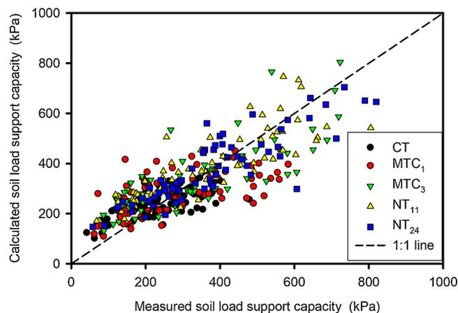
**Fig. 1.** Measured vs. calculated values of soil load support capacity under different tillage systems in a very clayey, Rhodic Eutrudox. Dashed line represents a one-to-one relationship.
