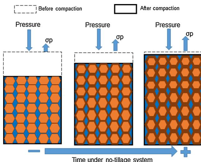
Fig. 4. Changes in the soil load support capacity ( $\sigma_p$ ) over time in no-tillage system due to age-hardening phenomenon.
