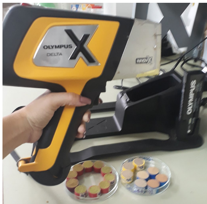
Figure 3: Portable X-ray fluorescence (pXRF) spectrometry device (Innov-X DP-6000 Delta Premium) analyzing ground Conilon coffee leaf samples collected in farms located in the north of the Espírito Santo state, Brazil.
