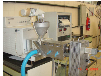
Figure 1. Digital photography of Brabender DSE 20 single screw extruder.
