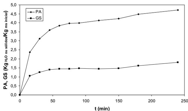
**Fig. 4** Water loss of and solid gain kinetics in the optimum condition of the osmotic dehydration of sweet potato slices. Source: Antonio (2006).
