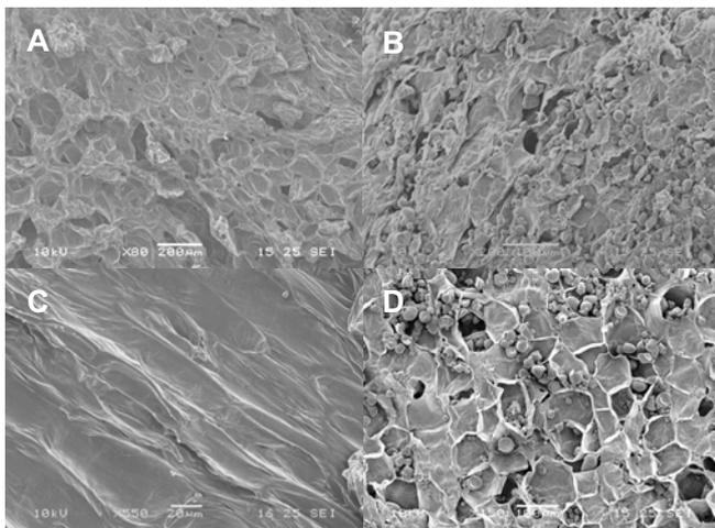
**Fig. 7** SEM images of the fresh sweet potato dried by HTST. (A) Surface - 110°C/5 min (X80); (B) core - 110°C/5 min (X200); (C) surface - 160°C/25 min (X550); (D) core - 160°C/25 min (X150).
