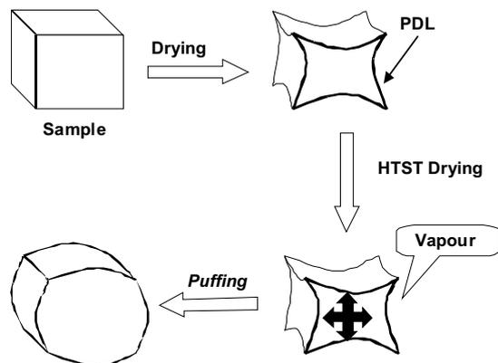
Fig. 6 Mechanism proposed for HTST drying. By GC Antonio.
