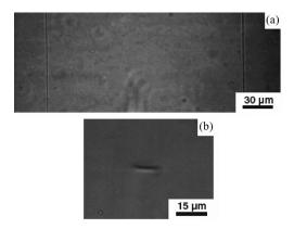
Fig. 6. (a) Optical microscope image of waveguides micromachined in PMMA doped with DR1 written at a speed of 20  $\mu$ m/s. (b) Cross section of the waveguides fabricated. Reprinted from [25]. Copyright [2008], with permission from Optical Society of America.
