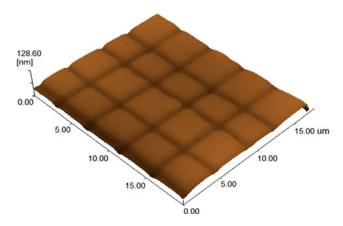
Fig. 8. Atomic force micrograph of a square-shaped-pillars morphology (4- $\mu$ m period) micromachined in PODR1 with 100-fs pulses and energy of 0.06 nJ.
