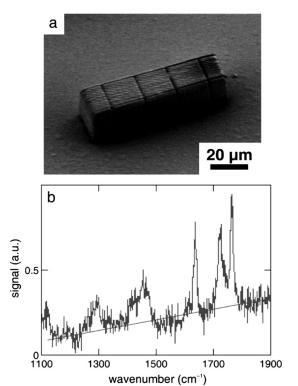
Fig. 12. (a) Scanning electron microscopy of a structure containing chitosan. (b) Raman spectrum of a two-photon polymerized microstructure doped with chitosan. Reprinted with permission from [78]. Copyright [2009], American Scientific publishers.
