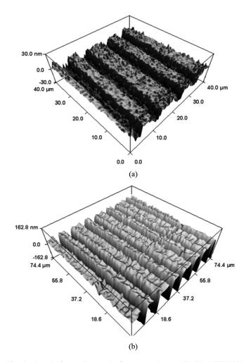
Fig. 4 Atomic force micrograph of grooves micromachined in MEH-PPV films with pulse energies of (a) 0.3 nJ and (b) 2.0 nJ. Reprinted from [46]. Copyright [2007], with permission from Elsevier.
