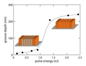
Fig. 5. Depth of the grooves as a function of the pulse energy for a translation speed of  $20~\mu\text{m/s}$ . The inset illustrates the two distinct micromachining regimes achieved. Reprinted from [46]. Copyright [2007], with permission from Elsevier.
