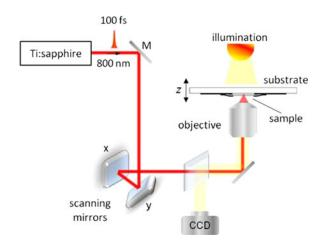
Fig. 3. Scheme of the experimental setup employed for the TPA polymerization.
