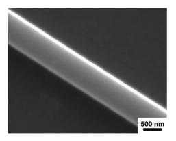
Fig. 15. Scanning electron microscopy image of a silica nanowire used to excite the fabricated polymeric microstructure.
