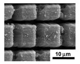
Fig. 9. Scanning electron microscopy image of PODR1 film microstructured with a period of 10  $\mu \rm m$ .
