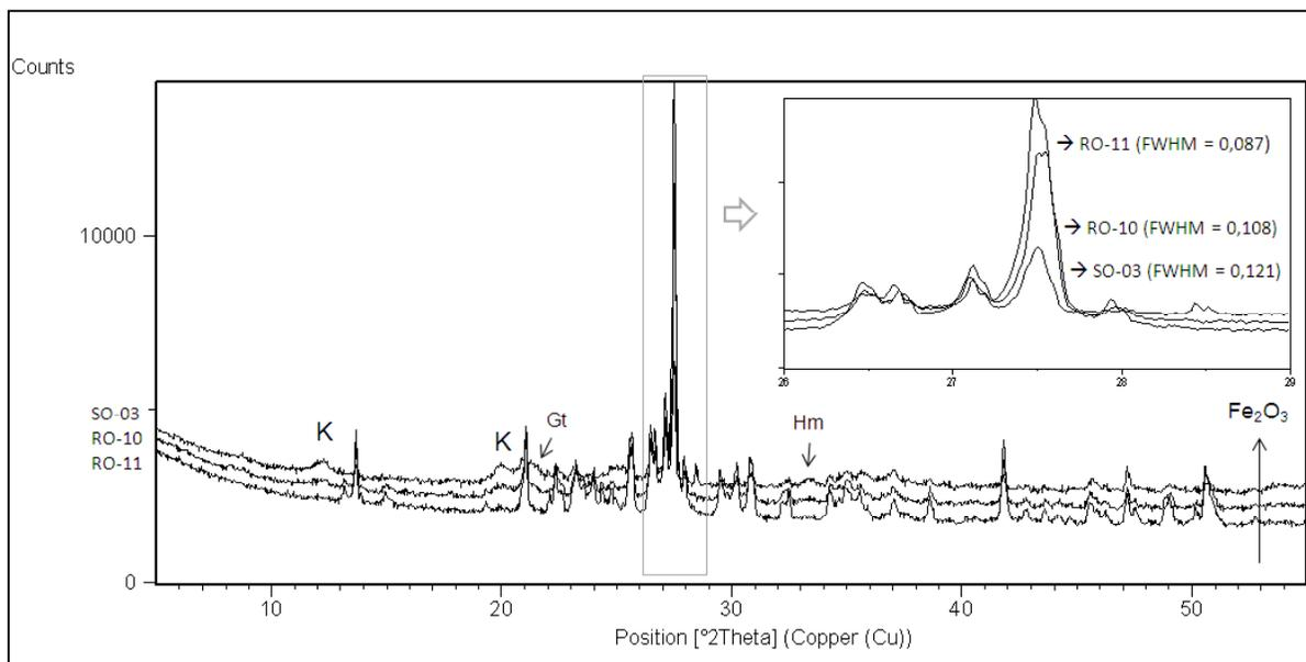
Figure 2. XRD patterns of the soil profile (three samples) from Figure 1, mainly composed by K-feldspar. In detail, one observes the K-feldspar most intense peak used for the FWHM measure and crystallinity evaluation. K: kaolinite; Gt: goethite, Hm: hematite.
