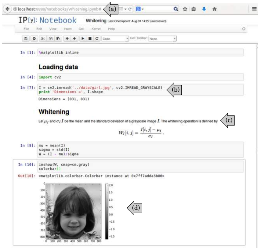
Figure 1. An IPython notebook. (a) IPython creates a Web server and users edit and manipulates their notebooks using a Web browser. (b) A code cell executes Python scripts. (c) A Markdown cell is able to present rich-formatted text and mathematical formulas using \text{\LaTeX} . (d) An inline plot using Matplotlib.
