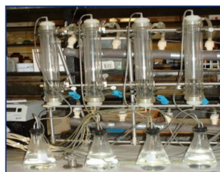
Figure 1. An accelerated temperature controlled incubation unit as described by Sartain et al. (2004). Credit: Luther Carson
