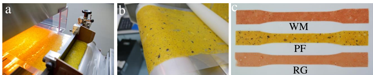
Figure 1: Illustrative photographs of continuous casting process for obtaining of fruit puree films. (a) Coating device, doctor knife type B, and IR predryer; (b) Rolling device and final fruit puree film; (c) Corresponding type I specimens for red guava (RG)-, passion fruit (PF)-, and watermelon (WM)-based films.
