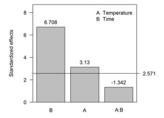
Figure 1. Pareto chart for the effects of temperature and time on the VOCs extraction.
