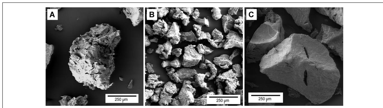
Figure 4—Scanning electron micrographs of soy protein isolates (SPI) prepared from hydrothermally treated soybeans at 100 $\times$  magnification: (A) control treatment; (B) SPI from 40 °C, 16 h-treated soybeans; (C) SPI from 60 °C, 16 h-treated soybeans.
