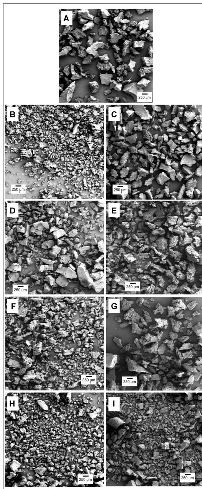
Figure 3—Scanning electron micrographs of soy protein isolates (SPI) prepared from hydrothermally treated soybeans at 20× magnification: (A) control treatment; (B) SPI from 40 °C, 4 h-treated soybeans; (C) SPI from 60 °C, 4 h-treated soybeans; (D) SPI from 40 °C, 8 h-treated soybeans; (E) SPI from 40 °C, 8 h-treated soybeans; (F) SPI from 40 °C, 12 h-treated soybeans; (G) SPI from 60 °C, 12 h-treated soybeans; (H) SPI from 40 °C, 16 h-treated soybeans; (I) SPI from 60 °C, 16 h-treated soybeans.
