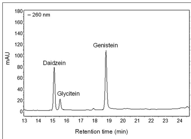
Figure 1—Mixture of isoflavones standard analyzed by high pressure liquid chromatography (HPLC).
