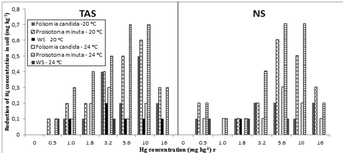
Fig. 1. Mean reduction of mercury concentrations in soils, in chronic reproduction tests with collembolans after 28 d of exposure, determined by Lumex RA-915+. TAS – Tropical Artificial Soil; NS – Natural Soil; WS – Treatments without collembolans.
