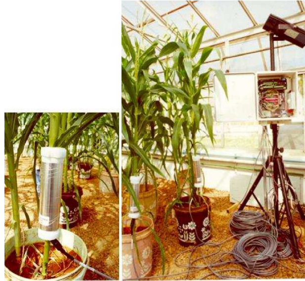
Figure 9. Energy balance probe (left) and automatic sap flow measurement system, installed on segments of eight maize ( Zea mays L. ) inbred lines plants stems for transpiration rate and water stress levels measurements at Sete Lagoas, MG, site (Embrapa Maize and Sorghum, Gomide et al., 2006).
