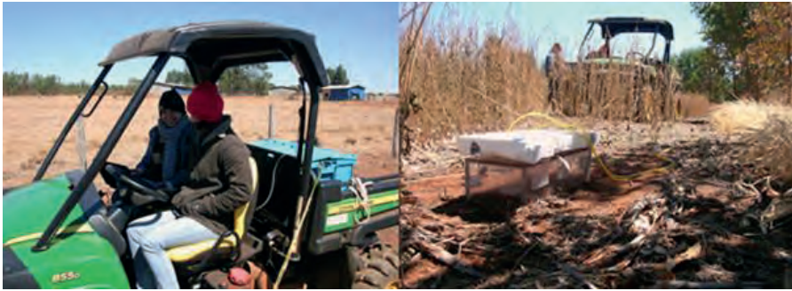
Fig 1. Chamber flux measurements at the soil-air interface in integrated livestock-plant system.
