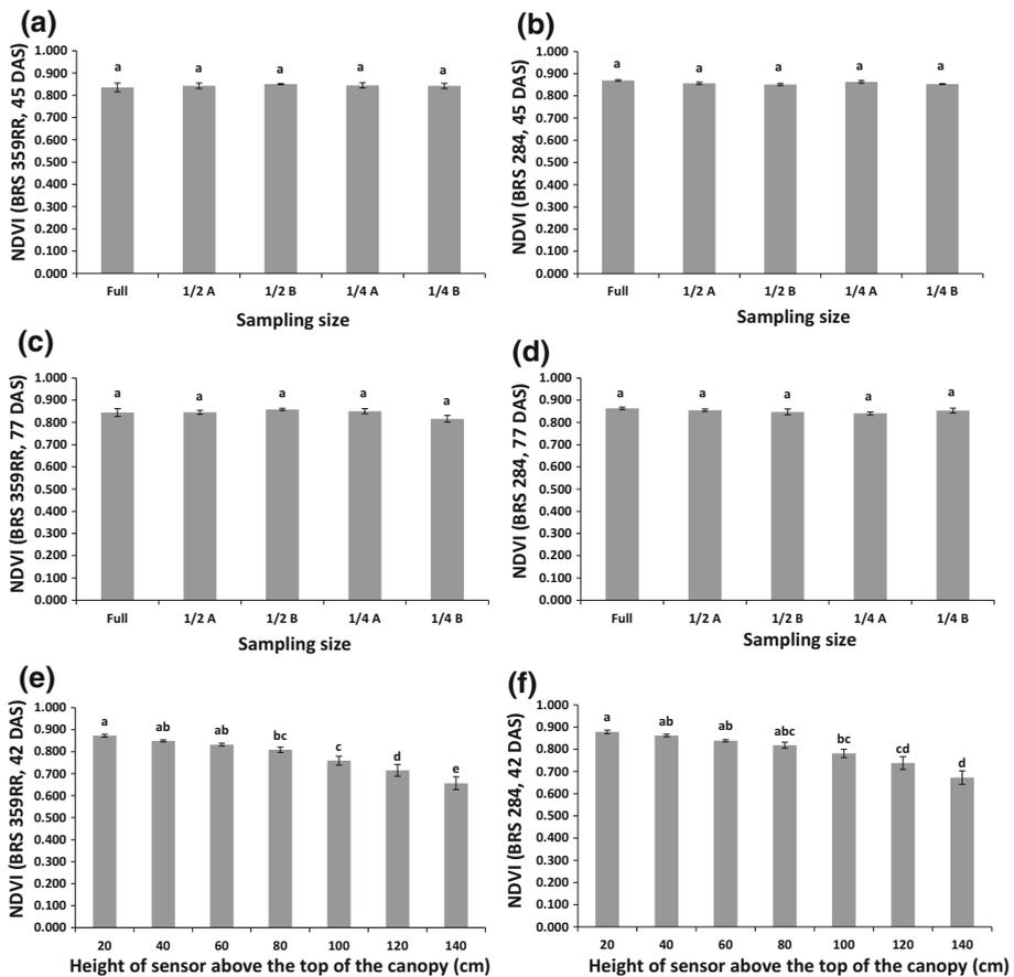
**Fig. 3** Values of NDVI in the soybean cultivars BRS 359RR and BRS 284 measured in different sampling sizes (a–d), and with the sensor positioned at several heights above the canopy top (e, f). Mean  $\pm$  standard error followed by the *same letter* do not differ by Tukey's test ( $p \leq 0.05$ ).  $n = 4$
