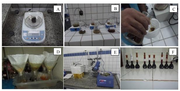
**Figure 1**. A) Weighing the crude propolis; B) Removal of the bioactive substances by shaking in grain alcohol; C) Filtration of the liquid phase; D) Filtered extracts; E) Concentration of the extracts in evaporator; F) Arrangement of the samples for extract color determination.
