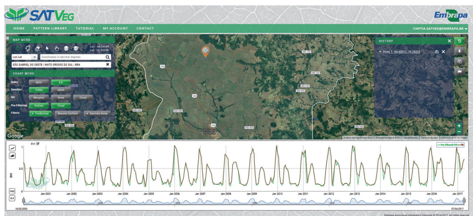
Figure 3 - Acquisition of MODIS pixels to evaluate the sowing and harvest period from the temporal profile of agricultural crops using SATVeg
