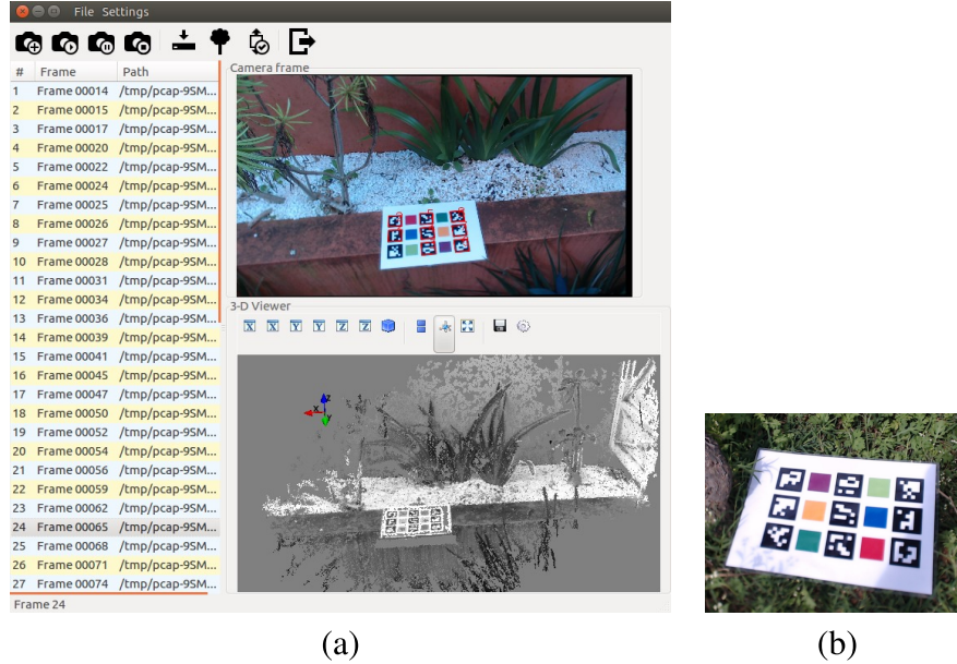
Figura 1: Screenshot of the 3-Demeter Capture application and the reference board. Application: (a - top) a camera frame where the board was found (the identified markers are highlighted in red); (a - bottom) the normalized 3-D point cloud (note the axis indicator). (b) The reference board with markers.
