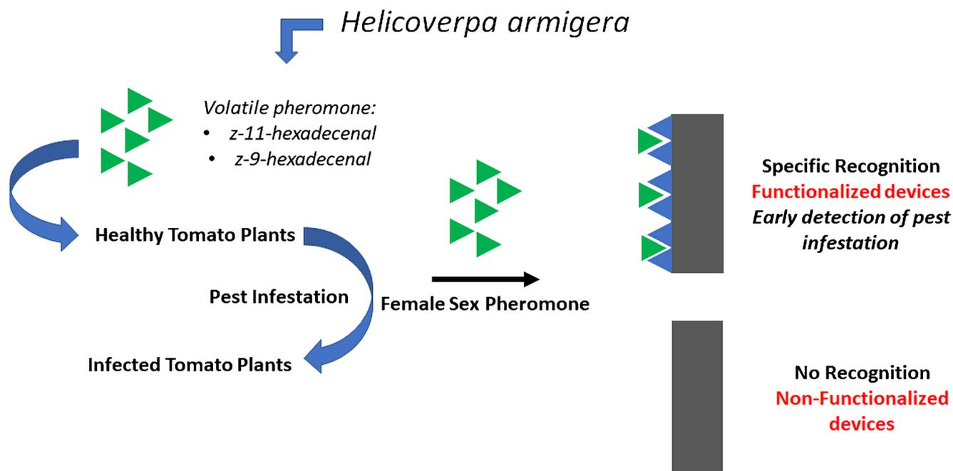
**Fig. 11** Photograph and schematic showing the use of a covalently functionalized MEMS device to detect female sex pheromones of *Helicoverpa armigera*, *Scirpophaga incertulas*, and similar pests prior
