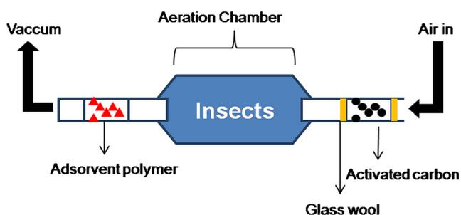
**Fig. 5** Schematic diagram of an aeration system used to collect insect volatiles for adsorption on a polymer
