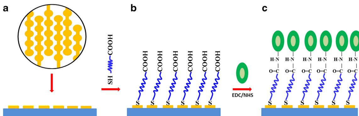
**Fig. 9a–c** Schematic of the immobilization of OBPs on poly(ethylene glycol)-modified interdigitated electrodes. **a** Interdigitated electrodes; **b** bonding of  $\alpha$ -thio- $\omega$ -carboxypoly(ethylene glycol) to the surfaces of the gold electrodes; **c** formation of covalent amino bonds between
