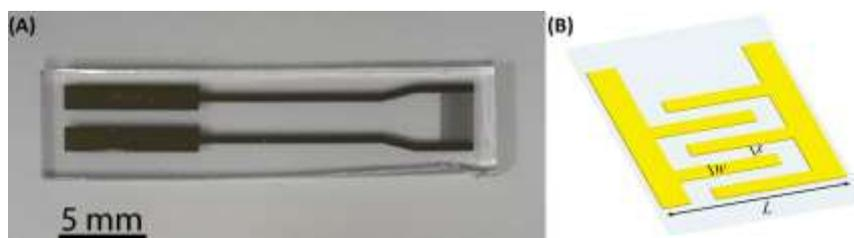
Figure A1: Digital picture (A) and a scheme of the geometrical features of the IDE (B). The fingers have a length ( $L$ ) of 4 mm and width ( $w$ ) and distance between fingers ( $s$ ) of 10  $\mu\text{m}$ .
