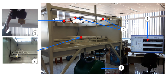
Figure 2. Development system for projects dedicated to the application of liquid agricultural inputs: (1) spray nozzle, (2) system that emulates the movement of the sprayer, (3) pesticide disposal tank, (4) user interface of the development system, (5) spray booms.
