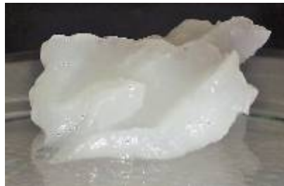
Figure 1: NC fibers (at 4%) dispersed in glycerin oil.
