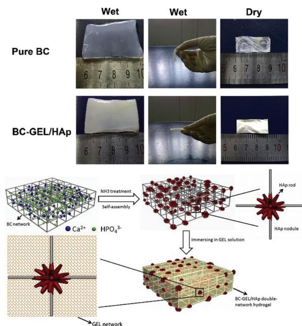
**Fig. 10** (Above) Digital photographs of the bacterial cellulose and bacterial cellulose/gelatin/hydroxyapatite composites in wet and dry states; (Below) schematic diagrams of the self-assembly of hydroxyapatite into the bacterial cellulose network and the preparation process of the double-network hydrogel.<sup>116</sup> Copyright 2017, Elsevier.
