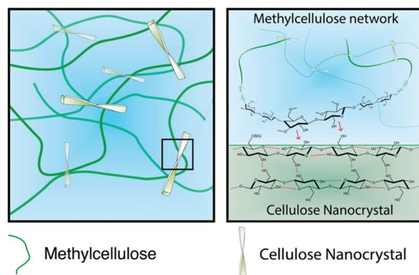
**Fig. 9** Schematic representation of the nanocomposite hydrogel. The suggested adsorption of MC on CNCs is indicated by red arrows.<sup>100</sup> Copyright 2014, American Chemical Society.
