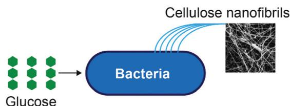
Fig. 4 Schematic image of bacterial cellulose production.
