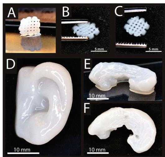
**Fig. 8** (a) 3D printed small grids (7.2 × 7.2 mm<sup>2</sup>) with 80% CNF and 20% alginate after cross-linking. (b) The shape of the grid deforms while squeezing, and (c) it is restored after squeezing. (d) 3D printed human ear and (e and f) sheep meniscus with 80% CNF and 20% alginate. Side view (e) and top view (f) of the meniscus.<sup>97</sup> Copyright 2015, American Chemical Society.
