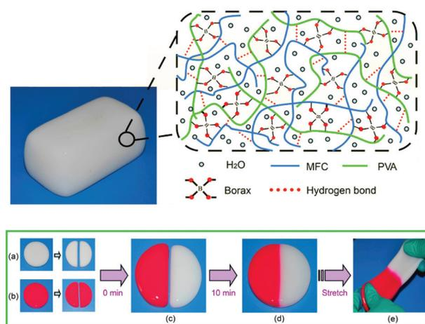
Fig. 12 (Above) Schematic illustration of the PVA/borax/CNF network and (Below) demonstration of the self-healing ability for PVA/borax/CNF at room temperature.<sup>131</sup> Copyright 2017, American Chemical Society.
