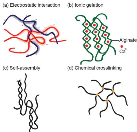
**Fig. 6** (a) Electrostatic interaction, (b) ionic gelation, (c) molecular self-assembly and (d) chemical cross-linking.
