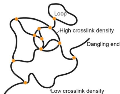
**Fig. 7** Hydrogel network defects.
