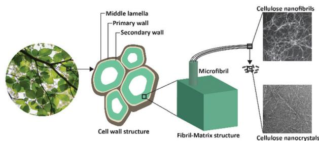
Fig. 2 Schematic representation of nanocellulose obtained from plants.
