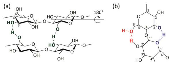
**Fig. 1** Chemical structure of cellulose. (a) Inter- and (b) intramolecular hydrogen bonds.
