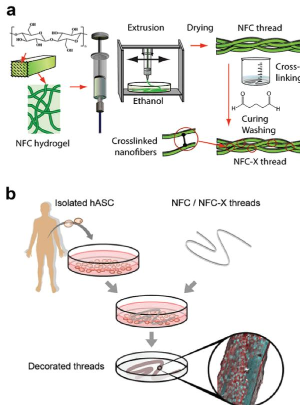
Fig. 15 Schematics for the preparation of NFC threads and their cross-linking with glutaraldehyde for NFC-X threads and (b) the process to decorate NFC and NFC-X threads with human adipose mesenchymal stem cells (hASC).<sup>148</sup> Copyright 2016, Elsevier.
