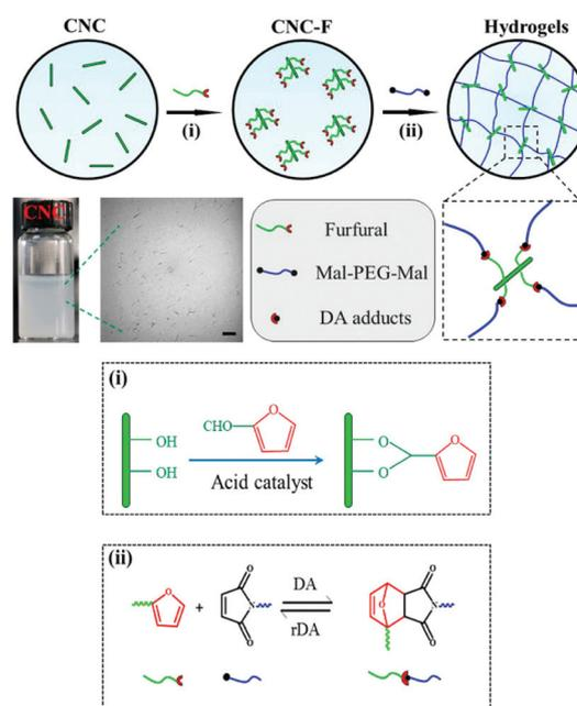
Fig. 13 Synthesis route to self-healing CNC-PEG nanocomposite hydrogels. Inserted images are the CNC aqueous solution and its TEM images, bar = 500 nm. (i) CNCs were modified with furfural by applying a well-known acetalization reaction in the presence of a solid acid catalyst. (ii) Reversible DA reaction between individual furyl and maleimide groups.<sup>135</sup> Copyright 2017, American Chemical Society.
