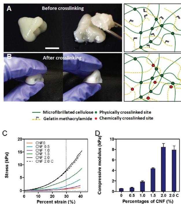
**Fig. 11** (a) 3D printed human nose structure before chemical cross-linking of gelatin methacrylamide (scale bar: 1 cm); (b) compressive test of a printed nose structure after cross-linking of gelatin methacrylamide; (c) compressive stress–strain curves and (d) compressive modulus of gelatin methacrylamide/CNF concentration composite hydrogels as a function of CNF concentrations.<sup>118</sup>
