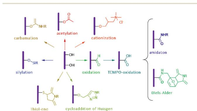
Fig. 3 Possible chemical modifications that can be conducted to cellulose.
