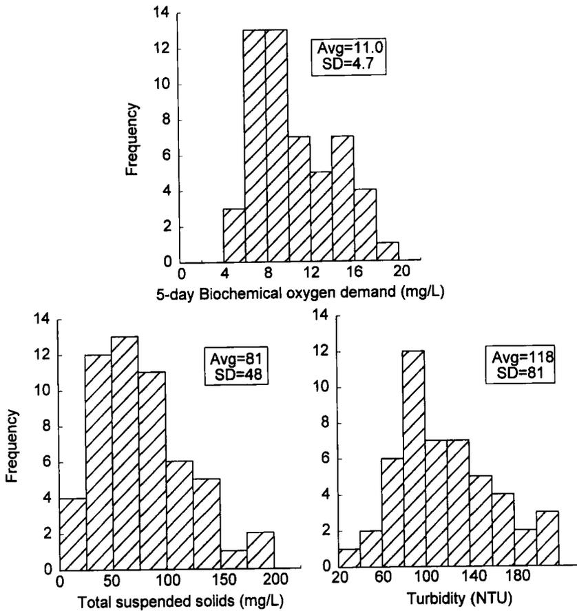
FIGURE 5. Concentrations of 5-d biochemical oxygen demand, total suspended solids, and turbidity in storm overflow from commercial channel catfish ponds in west-central Alabama.
