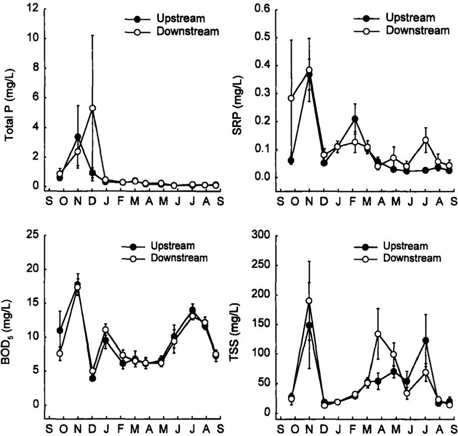
FIGURE 9. Averages ( $\pm$  SE) for concentrations of total phosphorus (TP), soluble reactive phosphorus (SRP), 5-d biochemical oxygen demand (BOD<sub>5</sub>), and total suspended solids (TSS) in eight streams at points upstream and downstream from channel catfish farming areas in west-central Alabama.
