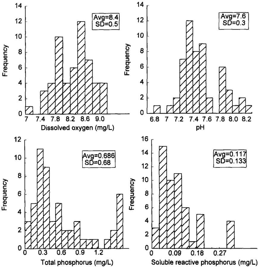
FIGURE 3. Concentrations of dissolved oxygen, pH, total phosphorus, and soluble reactive phosphorus in storm overflow from commercial channel catfish ponds in west-central Alabama.
