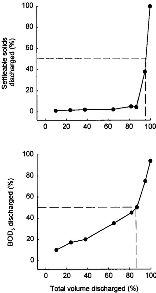
FIGURE 2. Percentages of settleable solids and 5-d biochemical oxygen demand (BOD<sub>5</sub>) discharged in relation to percentage of pond effluent discharged during draining of channel catfish ponds at Auburn, Alabama for harvest. Dashed lines indicate percentage of total pond volume discharged before 50% of BOD<sub>5</sub> and settleable solids loads were attained. Source: Schwartz and Boyd (1994a).
