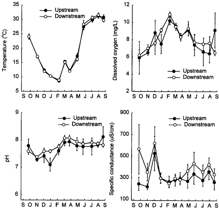
FIGURE 8. Averages ( $\pm$  SE) for water temperatures and concentrations of dissolved oxygen, pH, and specific conductance in eight streams at points upstream and downstream from catfish farming areas in west-central Alabama.
