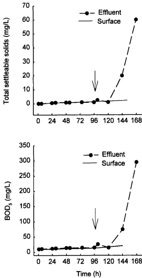
FIGURE 1. Concentrations of settleable solids and 5-d biochemical oxygen demand ( $BOD_5$ ) in pond surface water and effluent during draining of channel catfish ponds at Auburn, Alabama for harvest. Vertical arrows indicate time that harvest of fish began. Source: Schwartz and Boyd (1994a).
