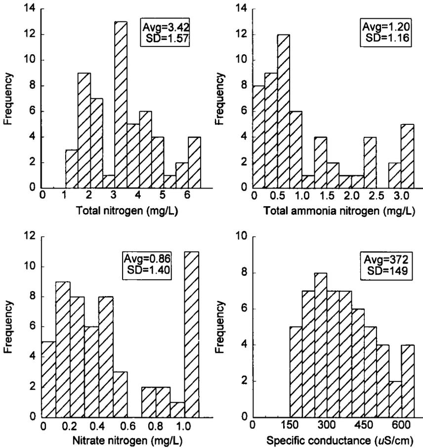
FIGURE 4. Concentrations of total nitrogen, total ammonia-nitrogen, nitrate-nitrogen, and specific conductance in storm overflow from commercial channel catfish ponds in west-central Alabama.
