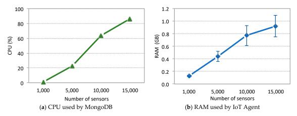
**Figure 13.** System metrics for the Guaspari Scenario: (**a**) CPU used by MongoDB; (**b**) RAM used by IoT Agent.
