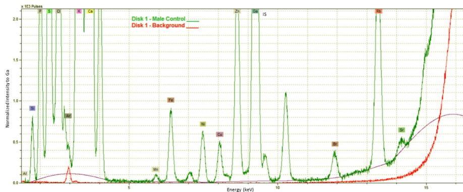
Fig. A.1. Spectra of male *Euschistus heros* hemolymph sample compared with the background reading, presenting the peaks of macro-elements and minor compounds. IS = Internal standard (Ga)
