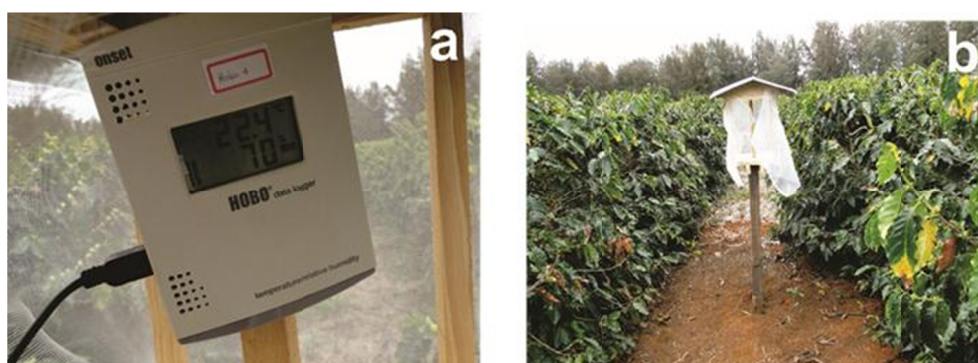
Figure 2. Temperature/Relative Humidity sensor (a) weather shelter (b)
