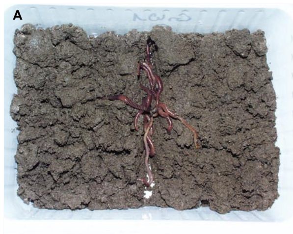
Photo 25.2. Design of the ISO Earthworm Avoidance Test. Two section design (A) and six section design (B). (Photo J. Römbke)
