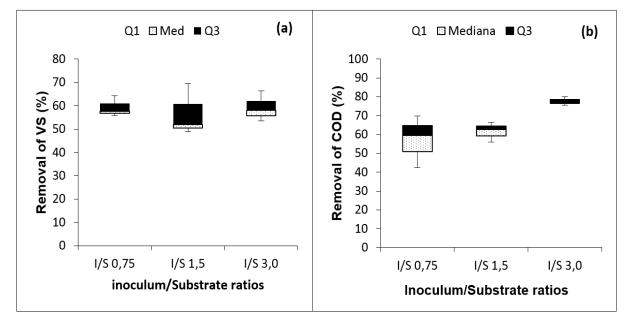
Figure 1. Organic removals in the different I/S relations. (a) Removal of VS. (b) Removal of COD.
