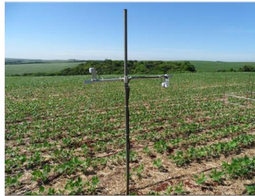
Figure 2. Incident (SRS NDVI Hemispheric) and reflected (SRS NDVI with Vision Limiter) radiation sensors installed in the experimental area. Carazinho/RS, 2017/18.
